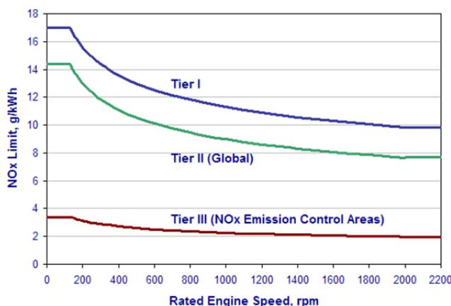
Figure 1 - MARPOL Annex VI NO<sub>x</sub> Emission Limits [www.dieselnet.com]
