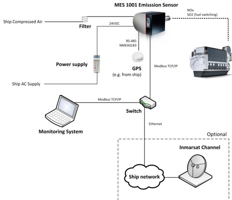
Figure 5 – Example of CEMS, Engine Control or Fuel Switching applications
