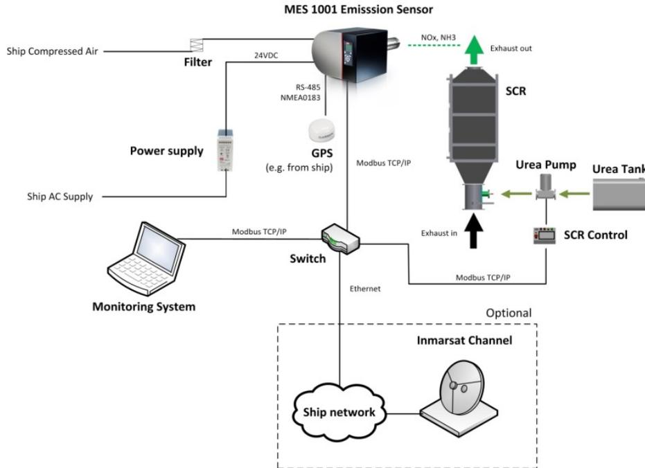
Figure 6 – Example of SCR Application
