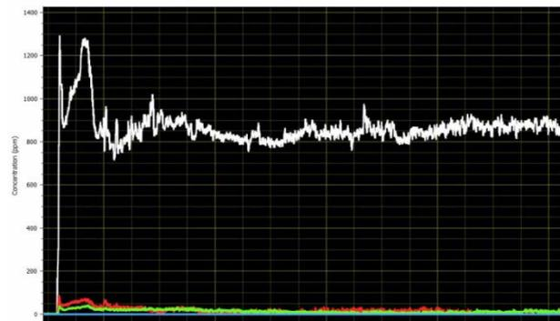
Figure 4 – Example of Measurement of NO (white), NO<sub>2</sub> (red) and SO<sub>2</sub> (green) over a 2-hour Period
